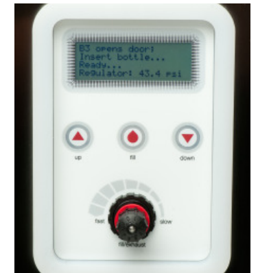
FIZZIQ Control Panel showing the screen, B1 (up), B2 (fill), B3 (down), and the Fill/Exhaust knob.
