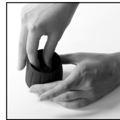
Fig. 10: Grasp valve with fingertips and remove
