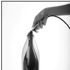
Fig. 6: Purge air from headspace for 3-5 seconds
