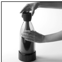
Fig. 7: Screw cap on with gentle force
